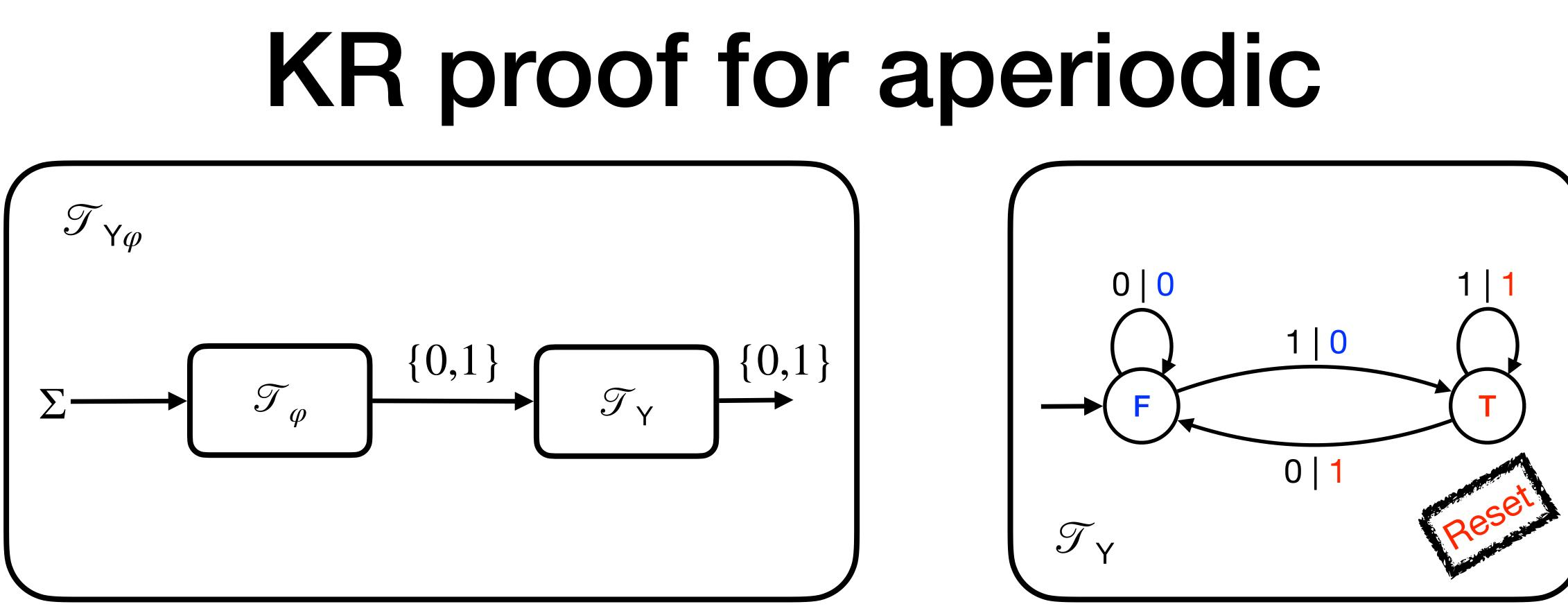
Given a PastLTL formula  $\varphi,$  we will implement  $\theta_{\varphi}$  with a transducer  $\mathcal{T}_{\varphi}$  constructed inductively as a cascade product of reset transducers. Example  $\varphi = Y a$
